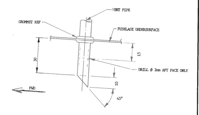
WING FUEL TANK VENT (MOD M701)
